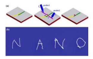
Nanoconstruction using nanoscale solder. (a) Touching nanowires can be joined using a nanoscale volume of solder melted from a sacrificial nanowire. (b) The word "NANO" written at the nanoscale by individual 55-nm-diameter gold nanowires. Adapted with permission from Nano Letters, ASAP Article, DOI:10.1021/nl8025339. Copyright 2008 American Chemical Society.
