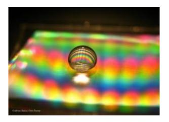
In the ultrasound sensor, the interface between water and air acts as a membrane. The vibrations of this membrane are measured using light.
