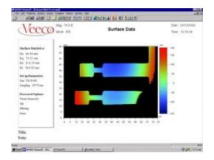
To compare different alloy compositions for their glass-forming ability, the researchers deposited slightly different blends of two metals on each one of an array of many microscopic fingers, or cantilevers, two of which are seen here, so that their properties could be compared side by side. Image courtesy / Carl V. Thompson
