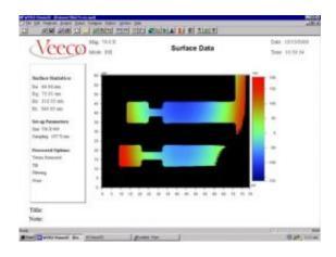
To compare different alloy compositions for their glass-forming ability, the researchers deposited slightly different blends of two metals on each one of an array of many microscopic fingers, or cantilevers, two of which are seen here, so that their properties could be compared side by side. Image courtesy / Carl V. Thompson
