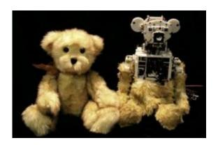
The Huggable robot, designed by researchers at the MIT Media Lab, was designed to enrich long-distance communication between users. Image credit: MIT Media Lab.
