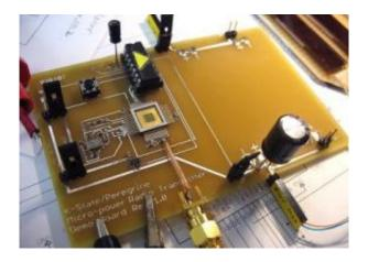
An in-progress demonstration board of an energy-harvesting radio developed at Kansas State University. The finished board includes solar cells to power the radio. Credit: Kansas State University
