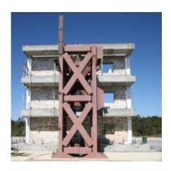
UC San Diego Engineers recently tested a 1920s era masonry building in order to design retrofit guidelines for such structures, which exist all over the world. Credit: UC San Diego Jacobs School of Engineering
