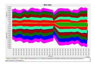
A sample of the results obtained at the Caltech booth at SC08, monitored by MonALISA, flowing in and out of the servers at the booth. The general smoothness of the TCP flows on the individual links is the result of using FDT. The feature in the middle of the graph is the result of briefly losing the local session at SC08 driving some of the flows.
