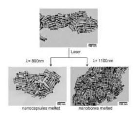
The top image shows a mixture of gold nanoparticles. The longer particles are called nanobones, and the smaller are nanocapsules. Bottom left: After the nanoparticles are hit with 800 nanometer wavelength infrared light, the nanocapsules melt and release their payload. Nanobones remain intact. Right: After the nanoparticles are hit with 1100 nanometer wavelength infrared light, the nanobones melt and release their payload. Nanocapsules remain intact. Image: Andy Wijaya
