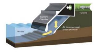
Schematic of an oscillating water column. Waves enter through a subsurface opening into the chamber with air trapped above. The wave action causes the captured water column to move up and down, pushing the trapped air into an electricity-generating turbine. The turbine turns continuously, despite the changing direction of the air stream as the waves come in and out. Graphic courtesy / MIT Energy Initiative
