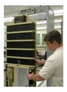
Guest researcher John Jendzurski prepares the NIST electromagnetic phantom for passage through the walk-through metal detector behind it. The carbonpolymer blocks of the phantom are arranged in a form that simulates the mass and height of the average American adult male. Metal objects such as the mock eyeglasses and belt buckle (top and center of the phantom) test the detector's function. Credit: Newman, NIST
