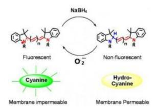
A new family of reactive oxygen species (ROS) probes -- called hydrocyanines -is synthesized by reducing a cyanine dye with sodium borohydride. Reacting with an ROS oxidizes the hydrocyanines into fluorescent cyanine dyes. Georgia Tech Image: Courtesy of Kousik Kundu
