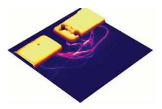
This 3D microscopic image of a simple nanotube device is taken with photothermal current microscopy performed in Jiwoong Park's lab. The two yellow blocks are electrodes, and strung between them are carbon nanotubes. The strength of each nanotube's electrical signal is visible according to its brightness. Image: Adam W. Tsen
