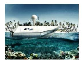
The Reefbot is relatively compact, autonomous surface craft designed to continuously collect data pertaining to the oceans' littoral zones, where most coral reefs are located.
