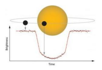
When the planet WASP-10b crosses the disk of its star, WASP-10, the brightness of the star decreases, allowing scientists to measure the precise size of the planet. Credit: Institute for Astronomy, University of Hawaii at Manoa
