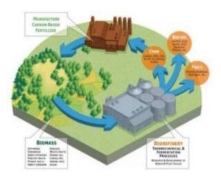
UGA's Biorefinery and Carbon Cycling Program, in partnership with EPRIDA, a private firm in Athens, Ga., host a pilot thermochemical biorefinery on the UGA campus. The pilot-scale refinery system converts peanut hulls to hydrogen (or other fuels) to biochar. This byproduct holds tremendous potential for carbon sequestration and production of soil amendments, bio-based products and fuels. Credit: University of Georgia
