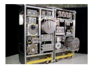
NASA&acutes new Water Recovery System will make it possible to double to six the number of crewmembers who can live aboard the International Space Station. Michigan Tech researchers helped optimize the design, increasing its efficiency by 30 percent. [NASA Marshall Space Flight Center (NASA-MSFC)]
