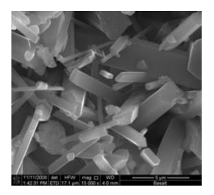
Shafts of calcite mineral grow rapidly on basalt after exposure to supercritical CO2 for 30 days. Use of dual beam focused ion beam scanning electron microscopy at the Environmental Molecular Sciences Laboratory helped capture the formation of the calcite. Image: PNNL
