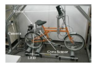
In the experimental set-up, the bicycle ran on rollers. The motor on the handlebars controlled steering, while the motor in the back drove the rear wheel. The gyro sensor, LED, and camera detected the bicycle's position, which gave feedback to a control system that adjusted the motors to maintain bicycle stabilization. Image credit: Yasuhito Tanaka and Toshiyuki Murakami. ©2008 IEEE.
