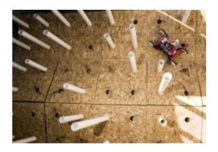
Robots are being trained to map spaces using their sensors. This robot travels through a simulated "wooded area" that has uneven terrain and randomly placed PVC pipes as "trees." It sends back data to researchers who use mapping algorithms to create a map. Credit: Texas Engineering Extension Service
