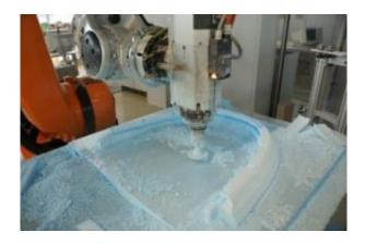
An industrial robot milling a mold for a large part. Credit: Fraunhofer IFF
