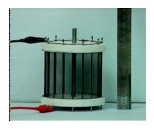
This paper-thin cylinder -- composed of carbon nanotubes -- emits sound in all directions. Credit: American Chemical Society
