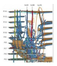
NIST graphic showing the buckling of WTC 7 Column 79 (circled area), the local failure identified as the initiating event in the building's progressive collapse on 9/11. Credit: NIST Building and Fire Research Laboratory
