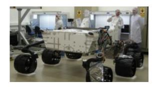
Wheels were first attached to NASA's Mars Science Laboratory rover in August 2008. The rover and its descent stage and cruise stage are being assembled and tested at NASA's Jet Propulsion Laboratory, Pasadena, Calif., for launch in 2009. Image Credit: NASA/JPL-Caltech
