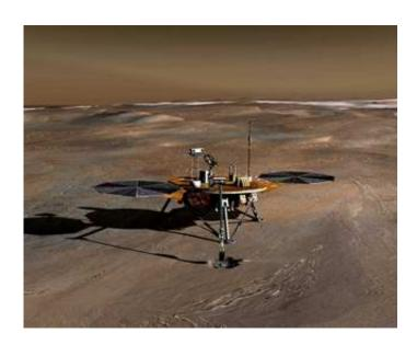
(PhysOrg.com) -- NASA's Phoenix Mars Lander has ceased communications after operating for more than five months. As anticipated, seasonal decline in sunshine at the robot's arctic landing site is not providing enough sunlight for the solar arrays to collect the power necessary to charge batteries that operate the lander's instruments.
