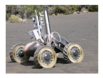
A prototype drilling rover built by Carnegie Mellon University carries RESOLVE, a small scale soil to oxygen conversion system. Its lunar wheels were developed by Michelin.
