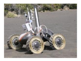
A prototype drilling rover built by Carnegie Mellon University carries RESOLVE, a small scale soil to oxygen conversion system. Its lunar wheels were developed by Michelin.
