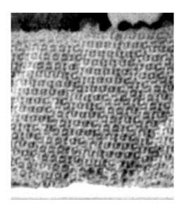
Scanning electron microscope photo of a thin film solar cell shows how the selfassembled gyroid structure interconnects in all directions, forming an easy path for current to flow out. Image: Wiesner Lab
