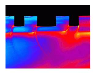
Close-up image of silicon microchannels. In microDMFC fuel cells, methanol and air circulate in microscopic microchannels etched in silicon wafers, as shown here. Image credit: Steve Arscott.
