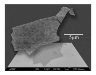
Two overlapping images of the same graphene sheet produced by hydrazine reduction; the top image was produced using atomic force microscopy, while the bottom was produced with scanning electron microscopy. This is the first reported instance of a graphene sheet being large enough for both tests to be run on the same specimen. (Image credit: Vincent Tung, Matthew Allen, Adam Stieg)
