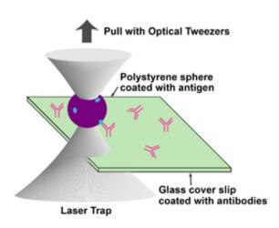
Basic scheme of an optical tweezer-based sensor of biological particles. A microsphere covered with a specific antigen (such as a virus or other infectious agent) is trapped and pulled away from a surface containing the corresponding antibodies. The minimum amount of force applied to the tweezers to break the bonds can provide information on the concentration of antibodies on the surface. Credit: NIST
