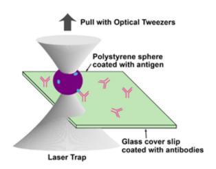
Basic scheme of an optical tweezer-based sensor of biological particles. A microsphere covered with a specific antigen (such as a virus or other infectious agent) is trapped and pulled away from a surface containing the corresponding antibodies. The minimum amount of force applied to the tweezers to break the bonds can provide information on the concentration of antibodies on the surface. Credit: NIST
