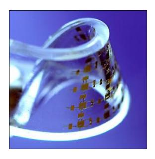
An optical image of an electronic device in a complex deformation mode.
