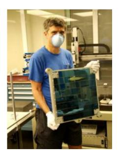
John Tonry of the Institute for Astronomy holds an entire array of 60 chips; an array of 60 OTAs will be installed in the focal plane of each of the four cameras in the Pan-STARRS facility. Photo / MIT Lincoln Laboratory
