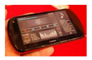
(PhysOrg.com) -- The dmedia G400 offers a choice of 3.8 or 4.3-inch touchscreen with an 800 x 480 resolution. The device features integrated WiMAX, Bluetooth, HSPDA/WCDMA, GPS, and a microSD card slot. Robust feature-sets enable bandwidth-intensive mobile multimedia applications that include NextWave's MXtv, mobile broadcast service, streaming video, video conferencing and VoIP.
