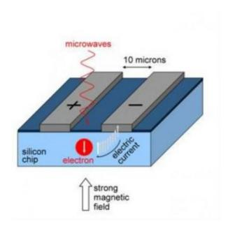
Microwaves are used to control the spin state of electrons held in silicon. This spin state can be watched in real time by measuring the electric current flowing between the (gray) electrodes. Credit: UCL/London Centre for Nanotechnology
