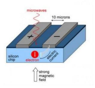
Microwaves are used to control the spin state of electrons held in silicon. This spin state can be watched in real time by measuring the electric current flowing between the (gray) electrodes. Credit: UCL/London Centre for Nanotechnology
