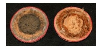
A cross-section of two cricket balls to illustrate the issue - the same brand, same model of cricket ball, but with two different cores. Left (darker core): rubber (extremely soft ball). Right: cork core (extremely hard ball). Photo courtesy of Dr Franz Konstantin Fuss.
