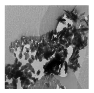
A transmission electron microscope image (magnified 5,000 times) of a slice of the Inti particle, which NASA's Stardust spacecraft collected in 2004 and returned to Earth two years later. Preparation of the sample caused some breakage. Scale bar is one micron, or one millionth of a meter. Image courtesy University of Chicago
