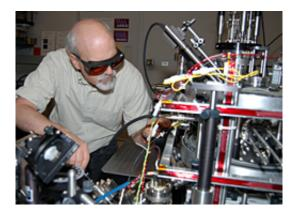
NIST researcher Jabez McClelland makes adjustments on the new magnetooptical trap ion source, capable of focusing beams of ions down to nanometer spots for use as a 'nano-scalpel' in advanced electronics processing. Credit: Holmes, NIST
