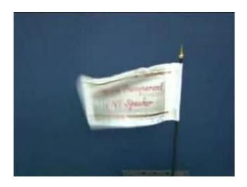
Excerpt from a video of Lin Xiao&acutes nanotube music speaker. The speaker produces sound when a current passes through, due to a thermoacoustic effect. Credit: Lin Xiao, et al.
