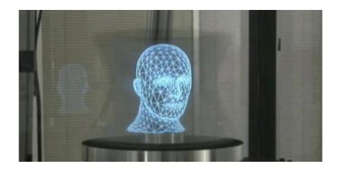
The 3D display system, developed by researchers at the University of Southern California, uses a spinning mirror to reflect images in all directions. Image credit: Graphics Lab at USC.
