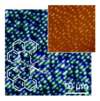
This spin-transition compound can be nanopatterned by unconventional and soft lithography to give crystalline, well-oriented, micrometer-scale structures arranged in stripes on a silica surface, as revealed by optical and scanning force microscopy (inset). (C) Wiley-VCH 2008
