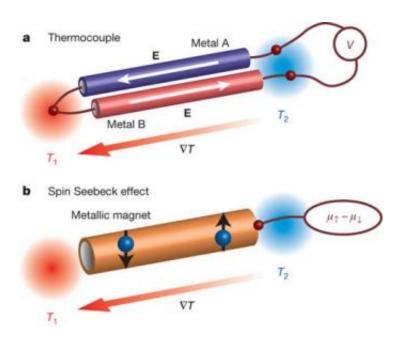
(A) Heating one side of a conductive rod causes heated electrons to move to the other end, creating a voltage. (B) Heating one side of a magnetized nickel-iron rod creates a "spin voltage," with spin-up and spin-down electrons on opposite ends. Image credit: (c)2008 Nature.
