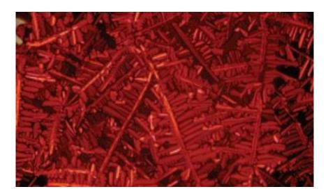
Polarized optical micrograph of a condensed porphyrin copper complex molecule with hydrophobic and hydrophilic side chains. Image credit: Tsuneaki Sakurai, et al.
