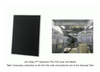
Sharp Corporation has completed installation of a new 2nd-generation thin-film solar cell production line at its Katsuragi Plant (Katsuragi City, Nara Prefecture) using large-size glass substrates measuring 1,000 x 1,400 mm, equivalent to 2.7 times the area of conventional substrates (560 x 925 mm), and will begin volume production this October.
