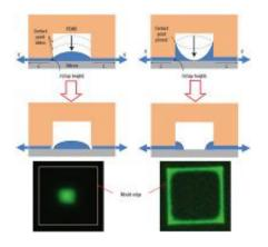
The thickness of the gap between a mold and the surface below determines how a drop of fluid will dry. A thin gap, left, lets the droplet pull away from the edges and shrink into a nanoscale structure. A thick gap, right, pulls the droplet toward the edges to form a "corral." Although the mold is a few microns across, the result is measured in nanometers, in a process developed by Cornell professor Dan Luo and colleagues. (Luo Molecular Bioengineering Lab)
