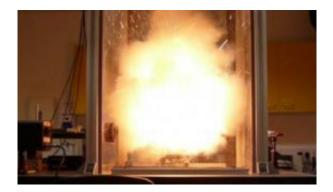
The detonation of a small pyrotechnic charge in the NPL facility. A radiation pyrometer on the left side of the image observes the event. Image: NPL
