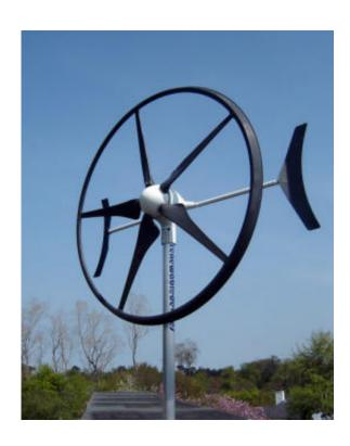
The Swift wind turbine, developed by the Scottish company Renewable Devices, was designed for quiet roof-top performance. Credit: Cascade Engineering.
