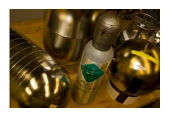
Different generations of collection cylinders used to collect air samples from locations around the world over the past 30 years. Scripps Institution of Oceanography at UC San Diego geochemistry researchers Ray Weiss and Jens Muehle led a study that found that the greenhouse gas nitrogen trifluoride, used in the manufacture of flat-panel monitors, escapes to the atmosphere at levels much higher than previously assumed. Credit: Scripps Institution of Oceanography, UC San Diego
