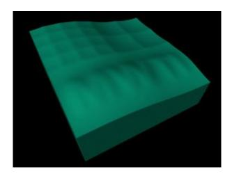
This freeform lens projects the ITWM logo: The upper half contains a negative image of the logo, while in the lower half you can see the letters ITWM as reversed as in a mirror. © Fraunhofer ITWM
