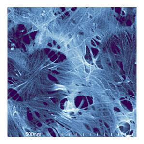
Buckypaper: SEM image demonstrates a pseudo 2-D network of carbon nanotubes deposited like paper fibers in a thin, sparse sheet. The nanotubes here have an average length 820 nm and make a continuous, electrically conducting network overall in spite of obvious gaps. On a macroscale this material would be nearly transparent. Color added for clarity. Image: Chastek/Talbott NIST
