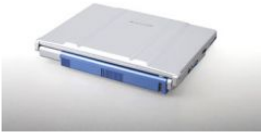
Panasonic Fuel Cell Prototype for Notebooks. Image: Panasonic
