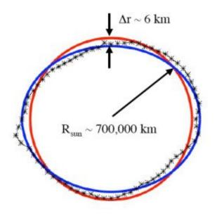
In this diagram, the sun's oblateness has been magnified 10,000 times for easy visibility. The blue curve traces the sun's shape averaged over a three month period. The black asterisked curve traces a shorter 10-day average. The "wiggles" in the 10-day curve are real, caused by strong magnetic ridges in the vicinity of sunspots.(NASA Goddard Space Flight Center)
